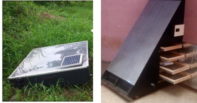
Fig.3.Fully constructed solar tunnel dryer and collector
